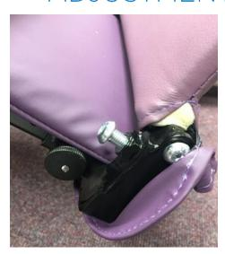
The Angle of the footplate can be adjusted using the chromed dome bolts, it is possible to adjust the angle from -10 degrees to +20 degrees.
